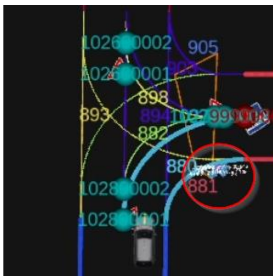
Figure 31. the pedestrian model accumulating too many pedestrians
