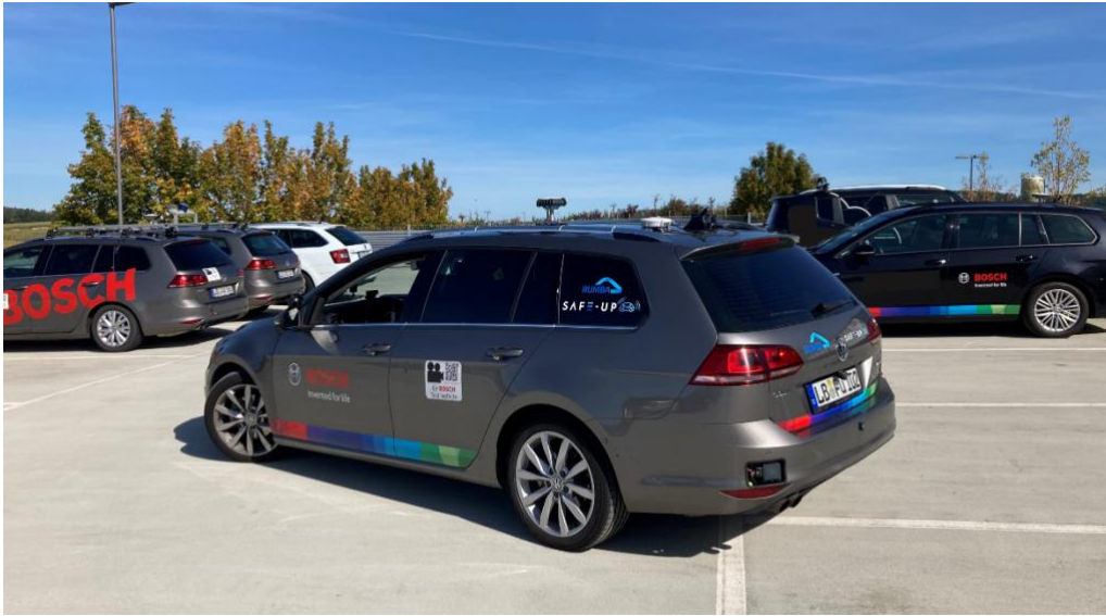
Figure 2: The Demo 3 vehicle : a Bosch development vehicle with close to series radar and video sensors.
