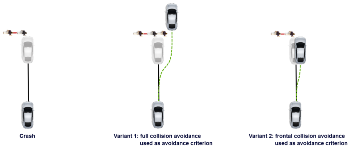
Figure 5: Avoidance criteria for the assessment of the accident/collision avoidance of an emergency steering or braking maneuver.
