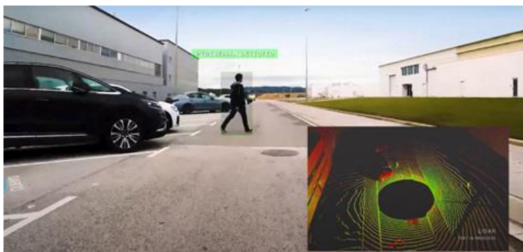
Figure 21: Preliminary test of the data fusion with on-board sensors
