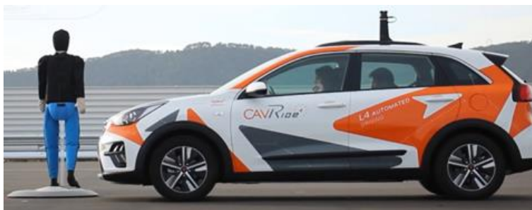
Figure 20: IDIADA CAVRide in a preliminary AEB VRU scenario
