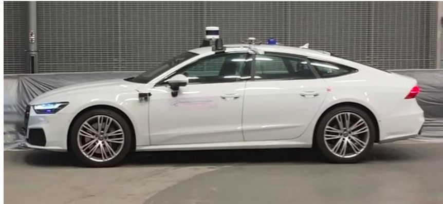
Figure 2: CARIAD development vehicle featuring a 360 degrees camera belt.
