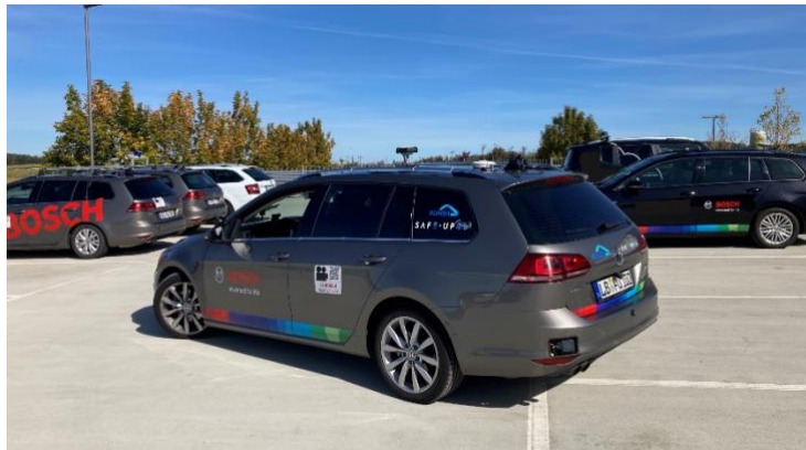
Figure 1: Demo 3 integration platform. A Bosch development vehicle featuring a radar/video sensor set and steering and braking interfaces with enhanced dynamics.
