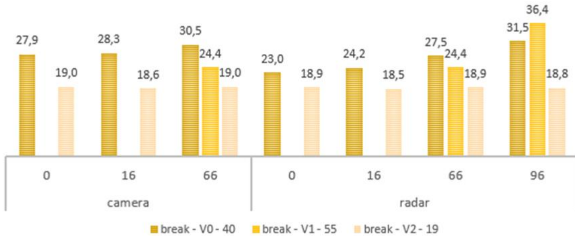
Figure 78: CPNAO – Collision speed depending on detection type and rain rate.
