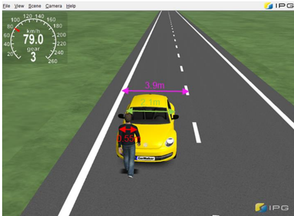
Figure 46: Definition of the different width, which are required for evasive steering.
