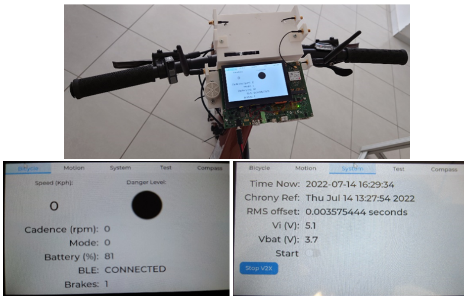
Figure 21: HMI example screens of VRU bicycle device.
