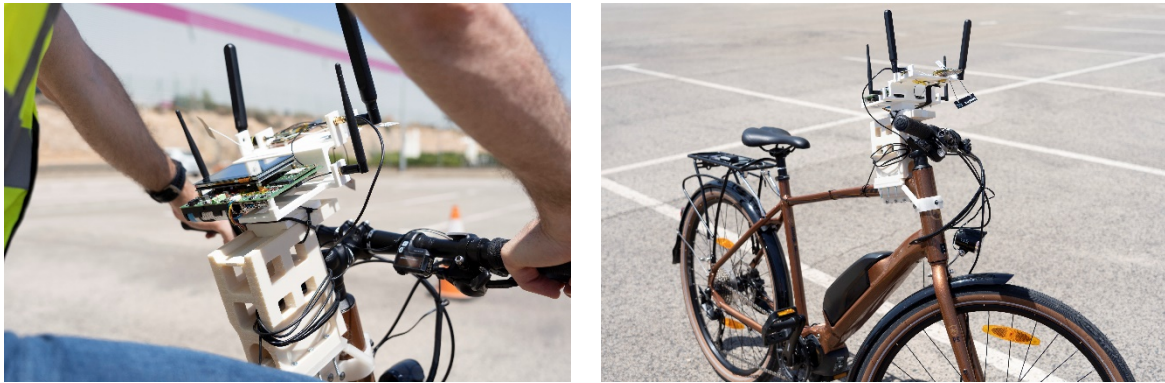
Figure 33: Views of the VRU device integrated in the bicycle for the testing phase at IDIADA premises.
