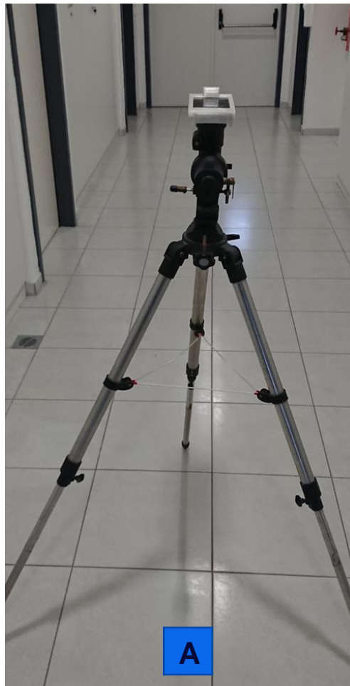
Figure 37: a) Orientation A (parallel to the ground)
