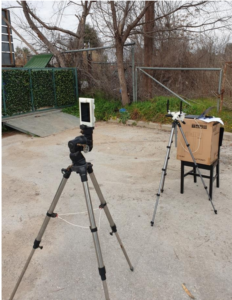
Figure 36: Photograph of the RF communication test configuration.
