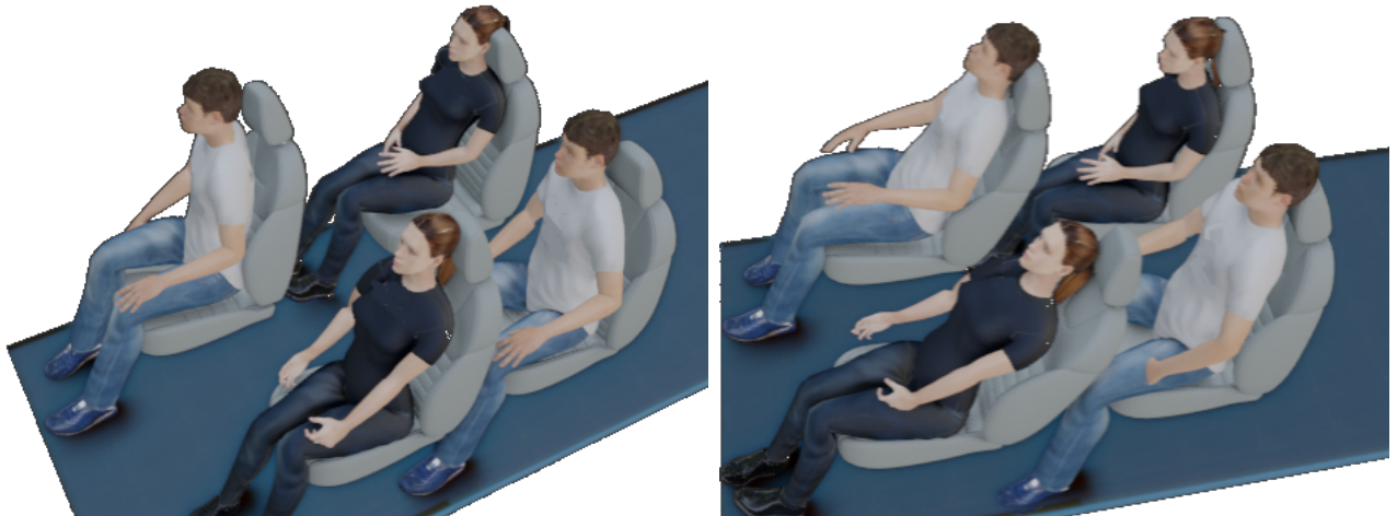
Figure 18. 3D view of SAFE-UP WP4 Peri-urban use case in Automation mode L3 interior configuration with increased legroom (left) or seatback recline (right)
