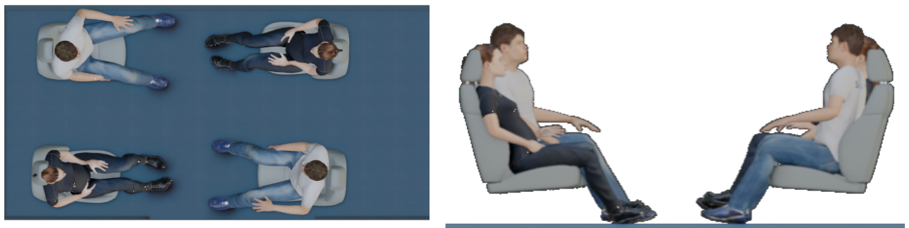
Figure 16. SAFE-UP WP4 Highway L4 use case interior vehicle configuration
