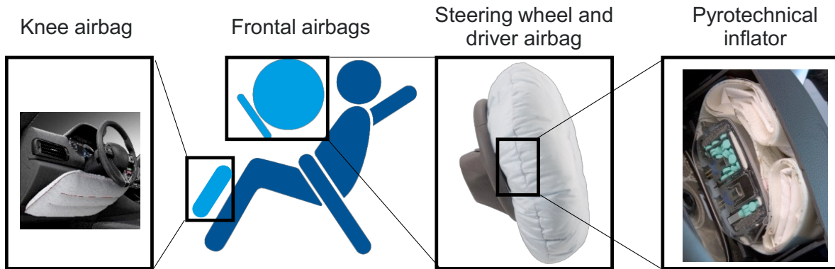
Figure 11.3 Frontal airbags in steering wheel and instrument panel.
