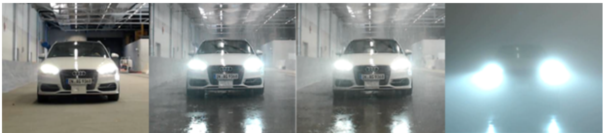
Figure 10 – Test vehicle under increasing bad weather conditions (THI)
