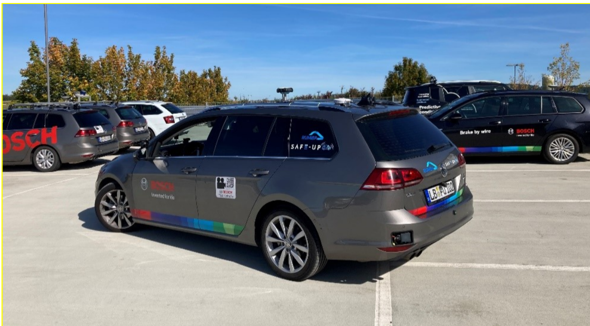
Figure 14 Demo 3 integration platform. A Bosch development vehicle featuring a radar/video sensor set and steering and braking interfaces with enhanced dynamics
