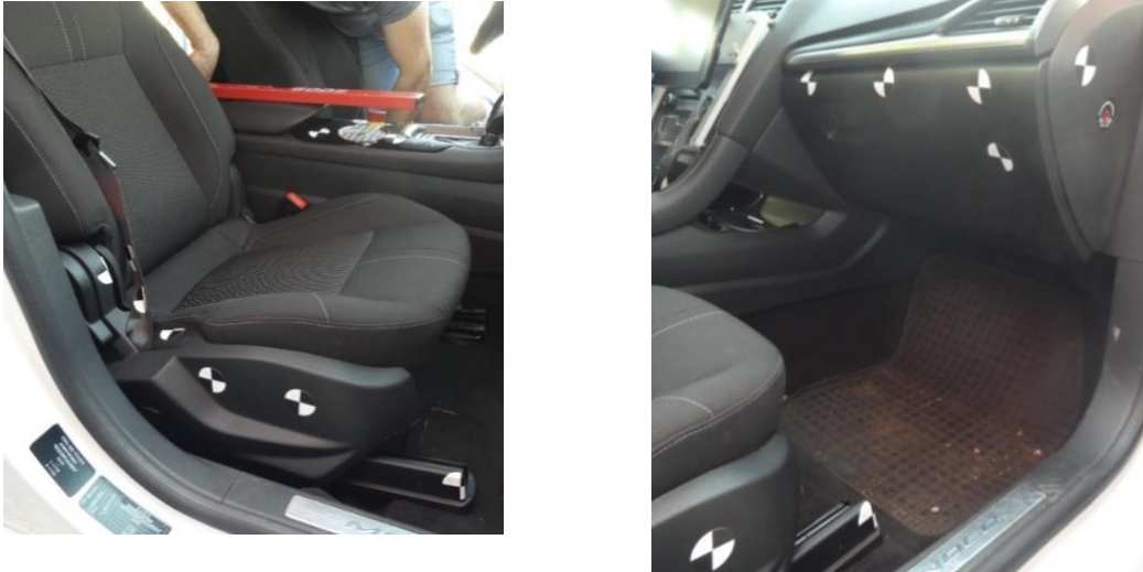
Figure 29: Vehicle interior with measured points
