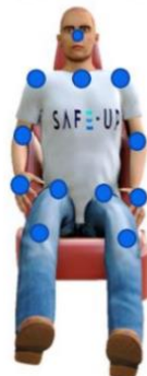
Figure 9: Output representation for pose estimation: body key points (blue circles)
