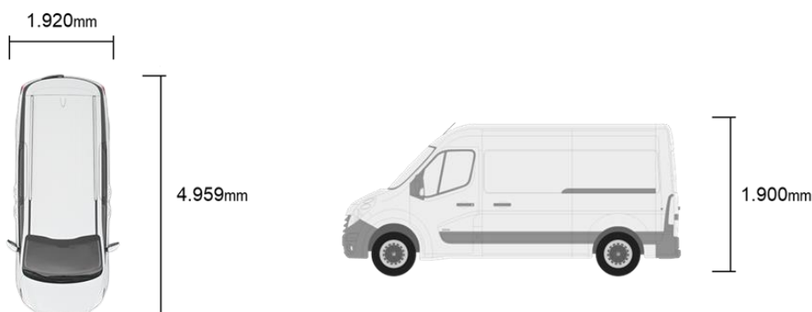
Figure 70. Dimensions of the large obstruction used for the Demo 4 cyclists scenarios
